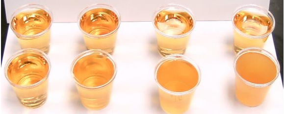
Figure 2. Corn in 0.3°B tea concentrate. From left: : 0.00%, 0.01%, 0.10%, 1.00%. Back row centrifuged at 3.7k rpm for 3min, supernatant.
